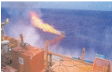
"Green burning" heavy crude oil during a full package DST-surface well testing job on the Nanhai-6 rig offshore China.
