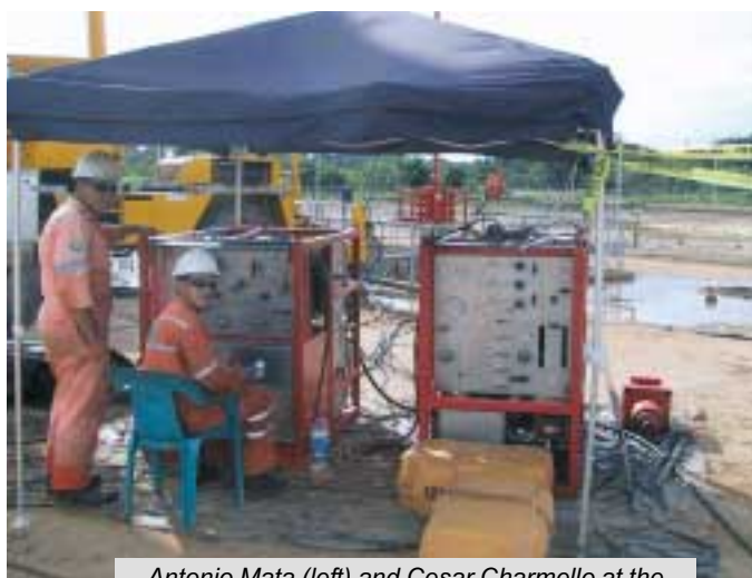
Antonio Mata (left) and Cesar Charmello at the control panels of 15,000 psi wire line pressure control equipment on site in Maturin, Venezuela.
